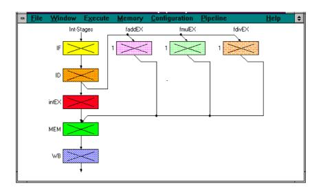
The picture shows the five pipeline stages of the DLX processor and the units for floating point operations (addition / subtraction, multiplication and division).
