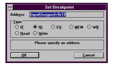
Now in the  $trap\ 0x5$ -line in the code window, "BID" appears, showing that a break from program execution will occur when this command is in the decode phase.
